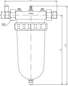
Screw-On Magnetic Filters Model MFR- Adapter Magnetic Filters Models MFT-I, MFT-A, MFT-L Flange Magnetic Filters Model MFF-
